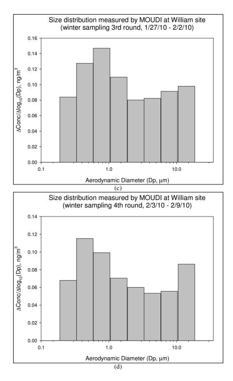
Figure 3. The ambient Cr-VI concentrations as a function of particle size by MOUDI sampling at William site within 50 m distant from the heavy trafficked NJTPK for the period of (a)  $1/13/10 \sim 1/19/2010$ , (b)  $1/19/10 \sim 1/26/10$ , (c)  $1/27/10 \sim 2/2/10$  and (d)  $2/3/10 \sim 2/9/10$ .
