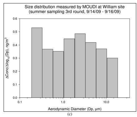
Figure 2. The ambient Cr-VI concentrations as a function of particle size by MOUDI sampling at William site within 50 m distant from the heavy trafficked NJTPK for the period of (a)  $8/4/2009 \sim 8/6/2009$ , (b)  $8/12/2009 \sim 8/14/2009$ , and (c)  $9/14/2009 \sim 9/16/2009$ .
