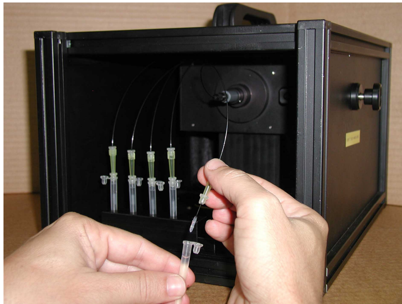
Fig. 5. Field-type portable photodetector device used at HMDC
