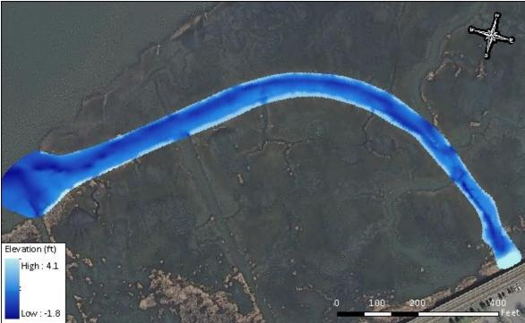
Figure 32 Anderson Creek, 1381 linear ft in length, branches from inlet on the Hackensack River curving to the back of the marsh where it quickly fades into a low marsh area then met with a wall supporting commuter rail lines. Average creek centerline elevation is -3.41 ft NAVD88. Minimum creek centerline elevation is -1.50 ft NAVD88 and maximum elevation is 0.70 ft NAVD88.
