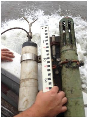
Figure 17 Sensor cluster from left to right: Sontek Argonaut 3 beam down looking ADV, CS451-L pressure transducer, YSI 6600 Multi-parameter Sonde
