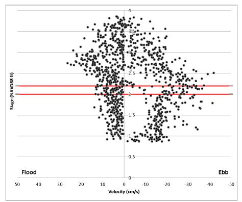
Figure 26 Anderson Creek: Sampled from 9/24/2014 – 10/8/2014, bank elevation: left 2.2 ft, right 2.0 ft. Peak flood velocity is seen above bankfull, peak ebb occurs at bank.
