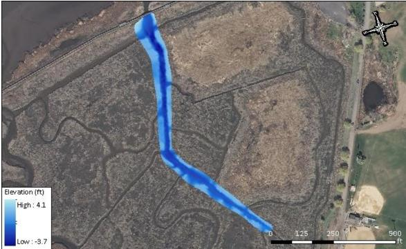
Figure 38 Secaucus High School Marsh Creek is 1453 ft in length with a minimum centerline elevation at -3.72 ft and maximum centerline elevation at 0.89 ft.
