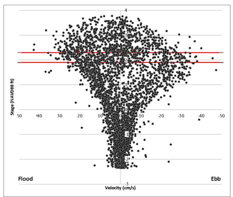
Figure 25 Secaucus High School Marsh: Sampled from 10/8/2014 – 11/5/2014, bank elevation: left 2.3 ft, right 1.9 ft. Peak flood velocity is seen above bankfull, peak ebb velocity occurs at bank.
