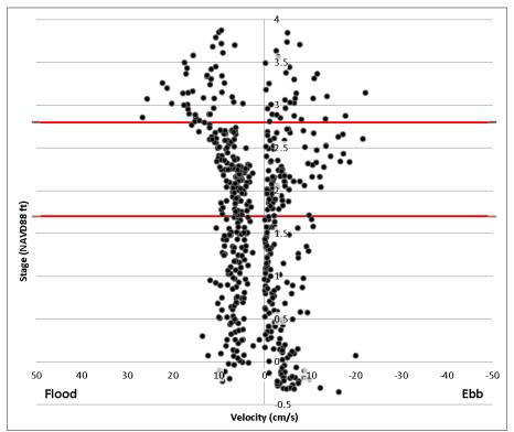
Figure 27 Hawk Property: Sampled from 8/1/2014 – 8/11/2014, bank elevation: left 1.7 ft, right 2.8 ft. Flood velocity dominant after overmarsh flow.
