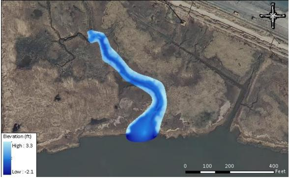
Figure 34 Fish Creek is the southernmost study site and is situated between the Hackensack River and active rail lines.. The creek is 711 ft in length with a minimum bottom elevation at -0.77ft and maximum at 1.73 ft.
