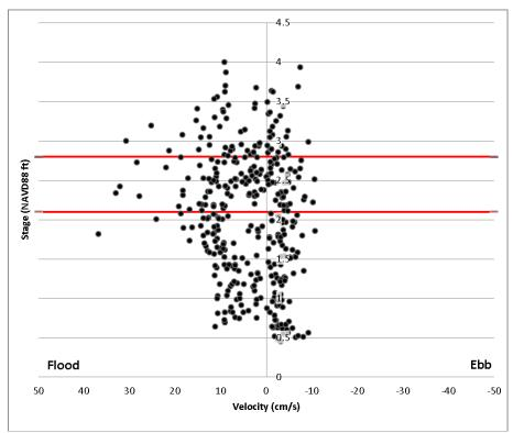
Figure 30 Bellemead Ditch: Sampled from 8/12/14 - 8/25/14, bank elevation: left 2.1 ft, right 2.8 ft. Peak flood velocity at 35 cm/s. Peak Ebb velocity occurs at the transition from overmarsh to undermarsh at 10 cm/s. Velocity is dominant during flooding.
