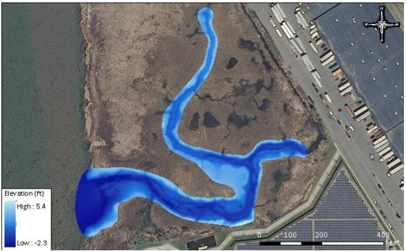
Figure 35 Hawk Property is positioned adjacent to the flow of the Hackensack River and surrounded by industrial and residential areas and a solar power array to the south. The primary creek is 1447 ft in length with a minimum bottom elevation at -1.9 ft and maximum at 1.2 ft.
